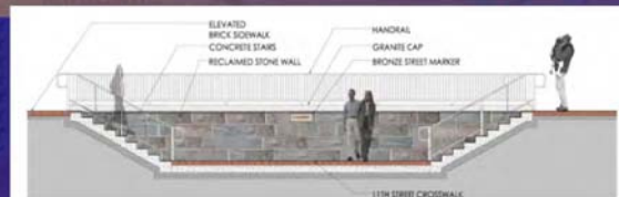
2 STAIRS AT 11TH STREET - SECTION/ELEVATION SCALE 1/4" = 1'-0"
