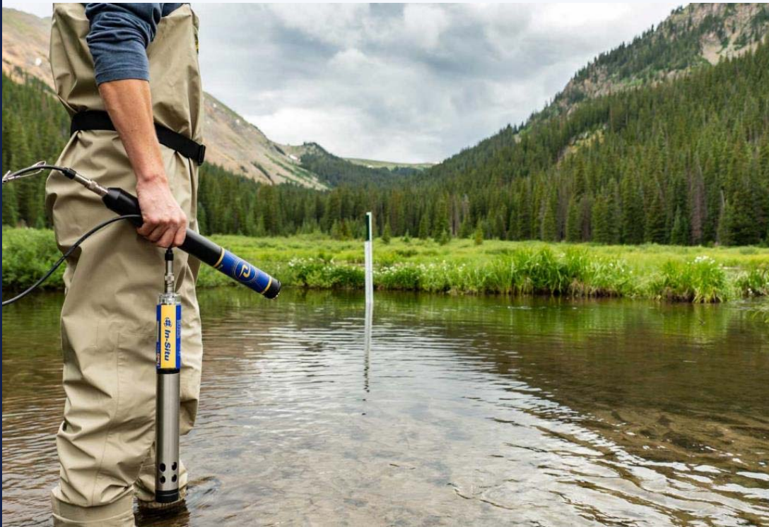
Cellular alert monitoring of dissolved oxygen and turbidity
