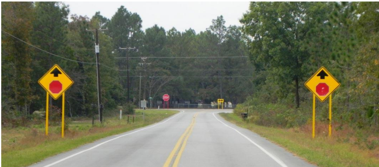
Figure 25: Advance Warning Signs & Pavement Markings. Source: South Carolina DOT
