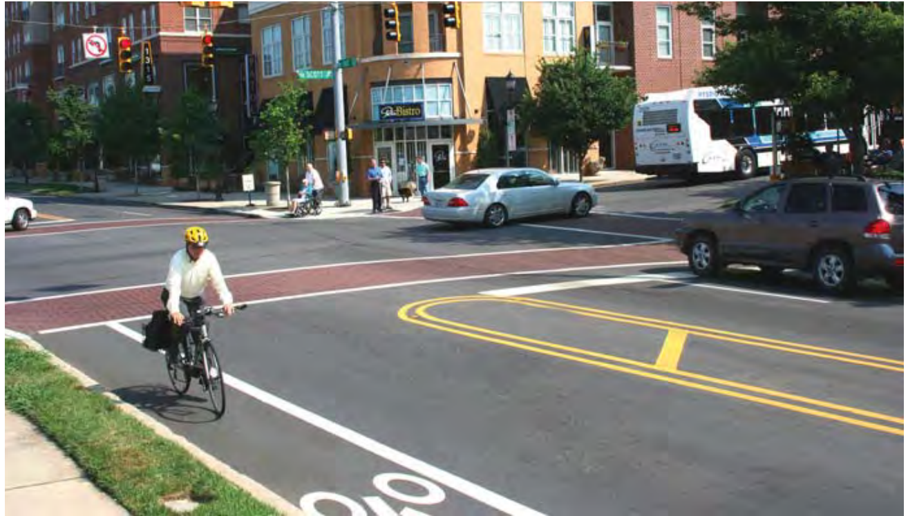
THIS IMAGE, FROM SMARTGROWTHAMERICA.ORG, ILLUSTRATES HOW COMPLETE STREETS PRINCIPLES WERE APPLIED TO AN INTERSECTION IN CHARLOTTE, NC
