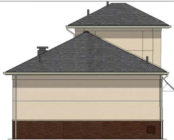
1 LEFT ELEVATION BRICK / EIFS
