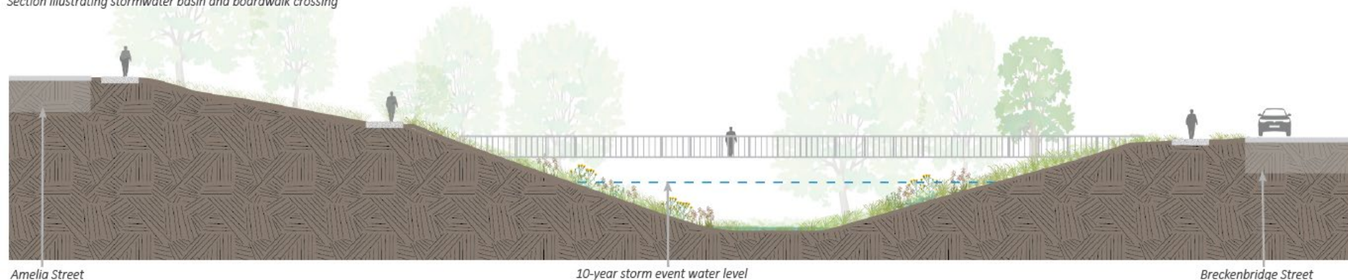
Section illustrating stormwater basin and boardwalk crossing
