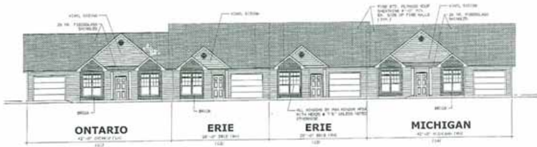
COMBINED SOUTH (FRONT) ELEVATIONS 1/8"=1'-0"
